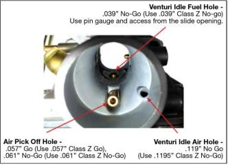
NOTE: Slide openings should be measured only with the Briggs & Stratton slide tool listed on the tool reference
